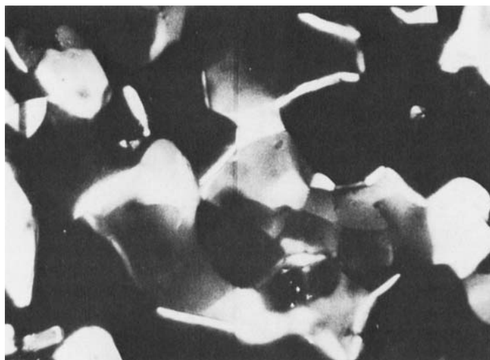
FIGURE 3 A smear of liquid n-butyl stearate on a glass slide cooled to the \alpha -phase showing some plane faces and sharp edges on the free surface, 26°C, crossed polarizers, 460 \times . There is no sample in some of the darker areas.
